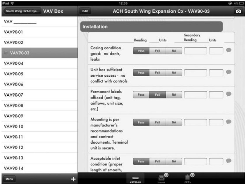
Figure 9-8. Commissioning on mobile tablets (TME 2013, unpublished).
