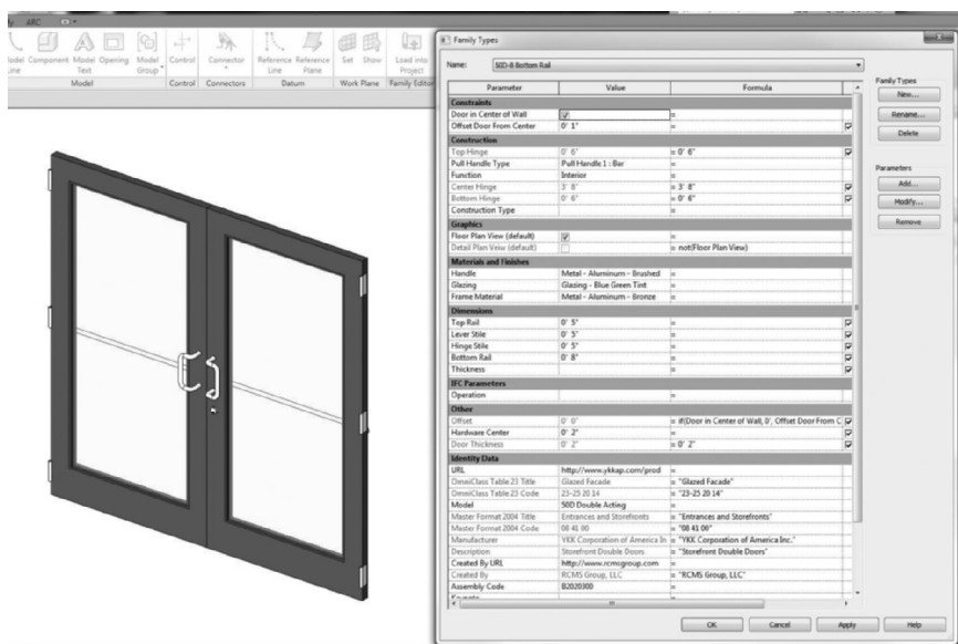
Figure 2.2 A door as a BIM object.
