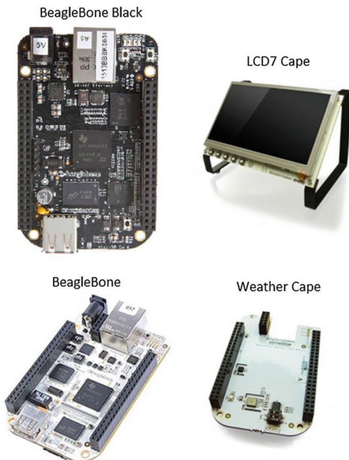
Fig. 4.3 BeagleBoard hardware and capes (BeagleBoard Web Site 2015). Source http://creativecommons.org/licenses/by-sa/3.0/legalcode
