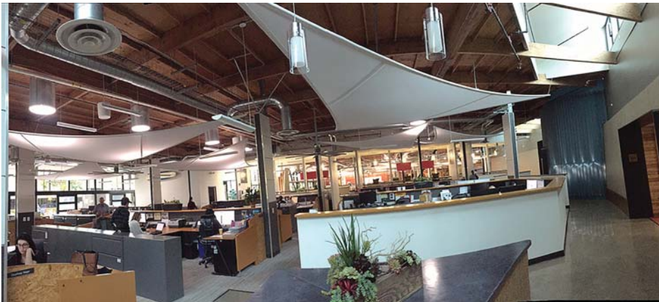
FIGURE 6.10 Natural lighting and sails with the electric lights off. © DPR Construction.
