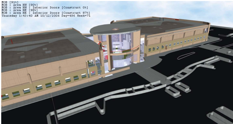
FIGURE 12.6 Screenshot of the construction sequencing of the PAMF Mountain View Center project. Courtesy of Sutter Health; courtesy of DPR Construction.
