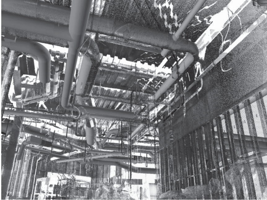
FIGURE 12.19 BIM superimposed over laser point cloud. Courtesy of Sutter Health; courtesy DPR Construction and Ghafari Associates, LLC.
