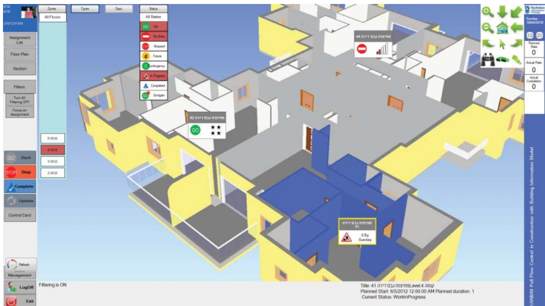
FIGURE 12.7 Drywall crew assignments in KanBIM. © Rafael Sacks, Associate Professor, Virtual Construction Lab, National Building Research Institute, Technion—Israel Institute of Technology.
