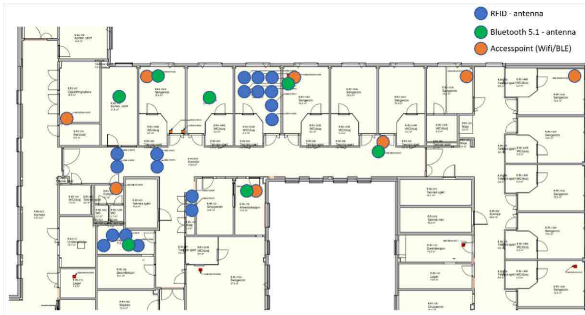
Figure 13: Proof of concept using automatic data capture technology to track movements and logistics
